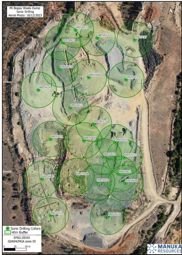
Figure 4: Sonic drilling and sampling (Left). Boppy Main Waste Rock dump sonic drilling Aol for each borehole, defining Indicated Resource areas (Right).
