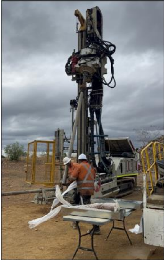
Figure 4: Sonic drilling and sampling (Left). Boppy Main Waste Rock dump sonic drilling Aol for each borehole, defining Indicated Resource areas (Right).
