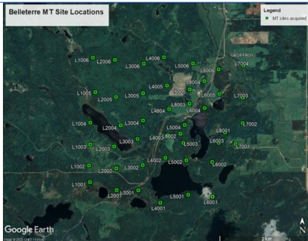
Figure. AMT points on seven lines surveyed by MoomBarriga GeoScience, 44 points.
