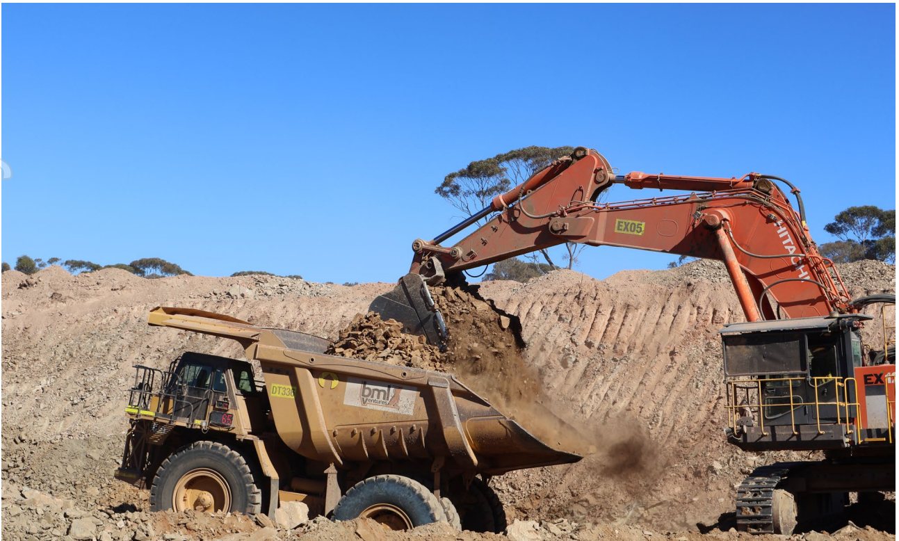
Ore being loaded onto a truck at Jeffrey's Find Gold Mine, Norseman.
