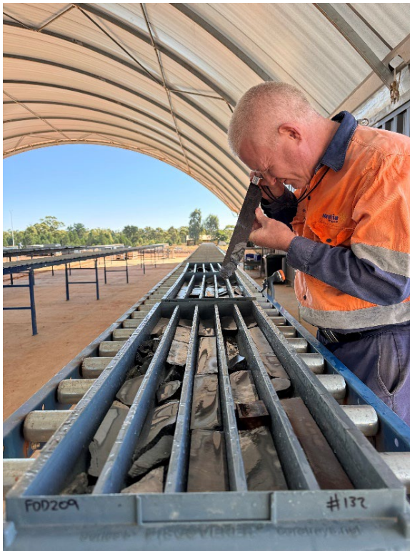
Figures 6 and 7: Senior Exploration Geologist Owen Thomas inspecting massive sulphides in drill core from FDD 209 @ 535.5m, and Drillcore photo from FDD209 with reported Zn grades in significant intersection 6m @ 27.2% Zn, 13.5% Pb, 0.3% Cu, 0.9g/t Au and 25g/t Ag from 534.0m.
