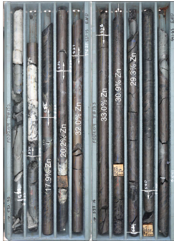
Figures 6 and 7: Senior Exploration Geologist Owen Thomas inspecting massive sulphides in drill core from FDD 209 @ 535.5m, and Drillcore photo from FDD209 with reported Zn grades in significant intersection 6m @ 27.2% Zn, 13.5% Pb, 0.3% Cu, 0.9g/t Au and 25g/t Ag from 534.0m.
