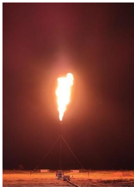
Flare (estimated to be 15 metres in height) from the Lorelle Sandstone Test at Daydream-2 during the 1 st flow period
