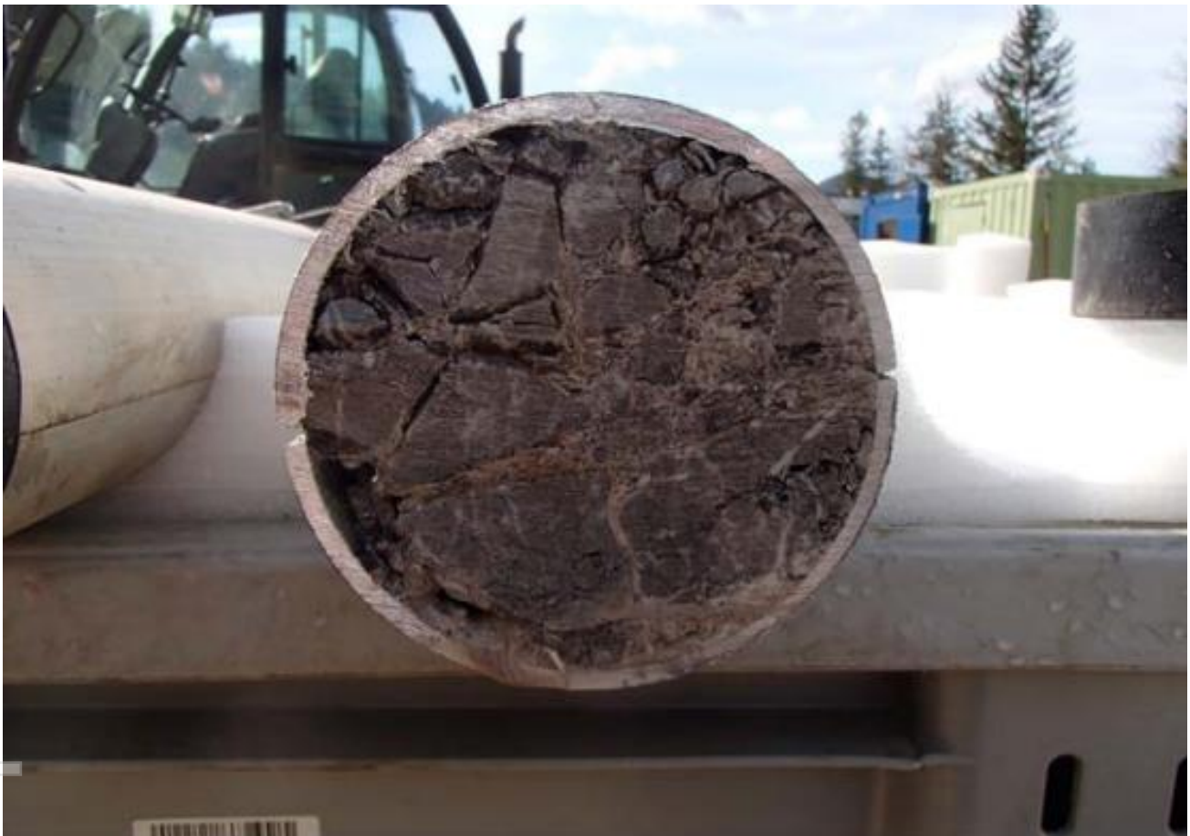
Cut section of Welchau-1 core demonstrating its natural fracture system
