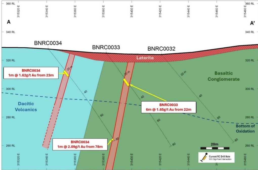
Figure Thirteen | Bouake North Cross Section of Drilling Testing New Gold & Arsenic Anomalism Along a Lithological Contact
