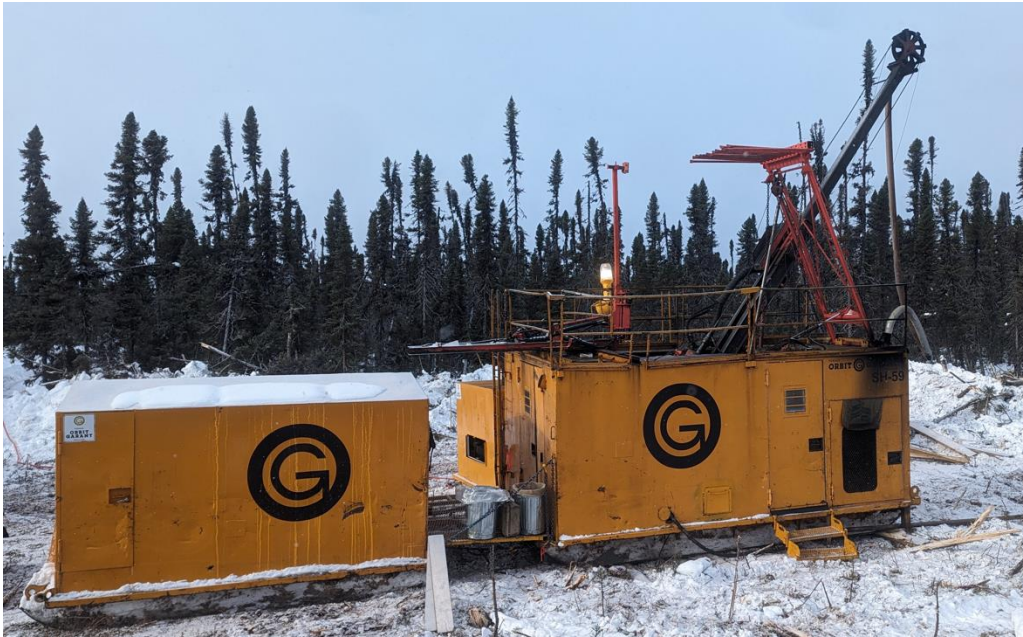
Figure 2: Diamond drill rig at Horden Lake project
