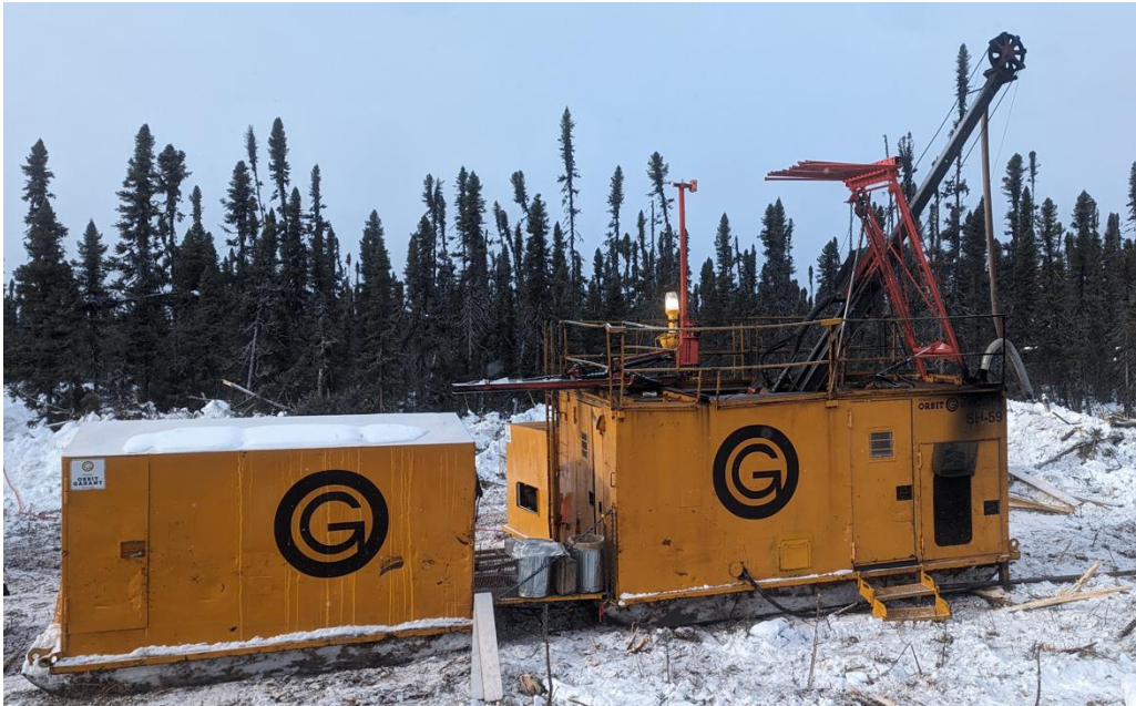
Figure 2: Diamond drill rig at Horden Lake project
