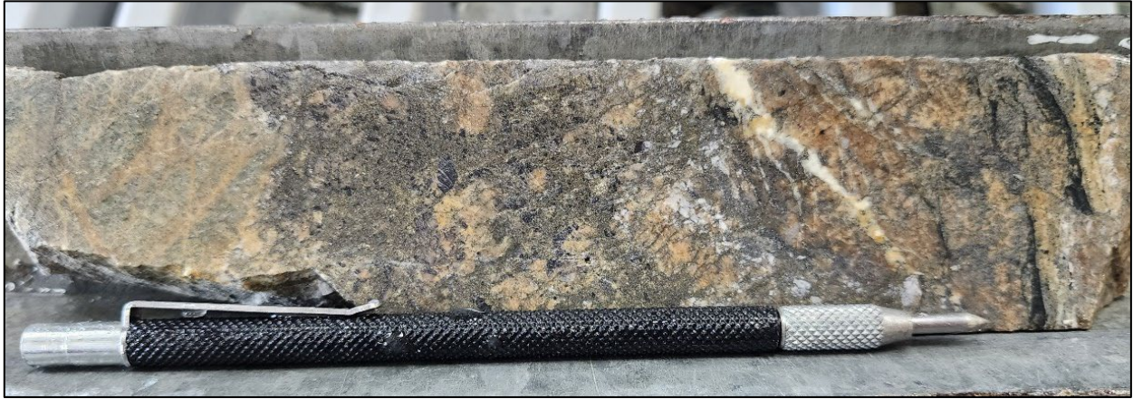
Figure 6: Mineralised carbonate-pyrite-arsenopyrite-cobaltite-scheelite vein (2019FTD007E, 129.8m) (Interval 129.5-130.0m Assay: 0.5m @ 6.64g/t Au, 0.38% Co, 1.02% WO 3 , 0.11% Cu ).
