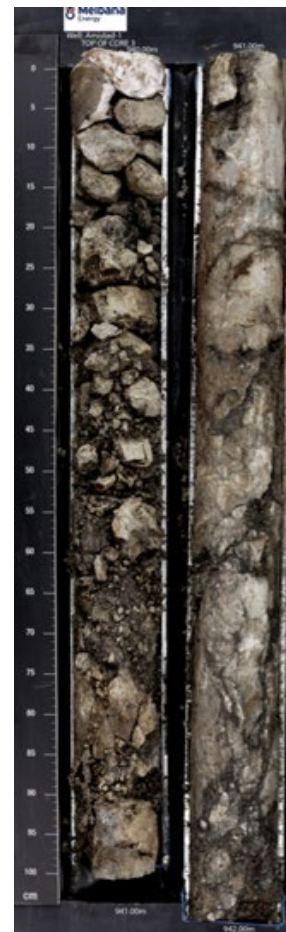
Figure 2 – Oil filled and heavily fractured limestone from Unit 1B
