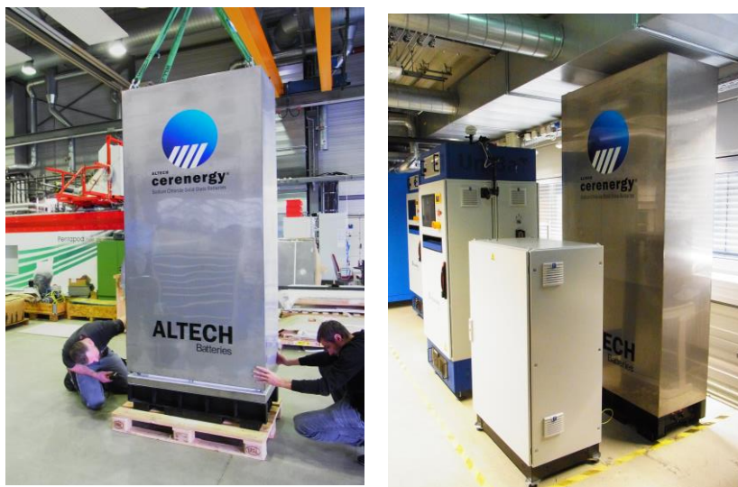
Figure 31 - Delivery of the battery casing and heat loss testing at Fraunhofer IKTS Dresden
