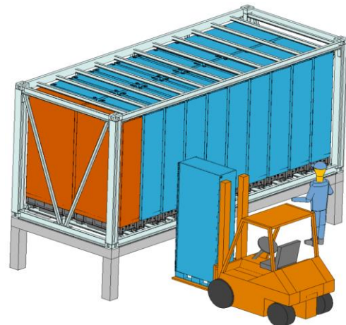
Figure 25 – Assembly 1 MWh GridPack
