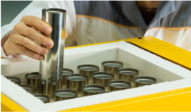
Figure 3 – CERENERGY® cells in battery module
