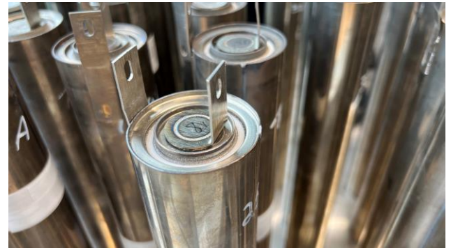
Figure 6 – CERENERGY® cell with positive and negative terminal
