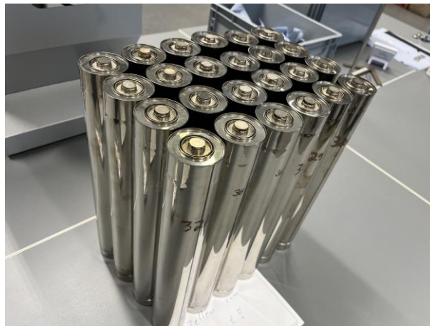
Figure 30 – Some of the completed battery cells waiting performance testing
