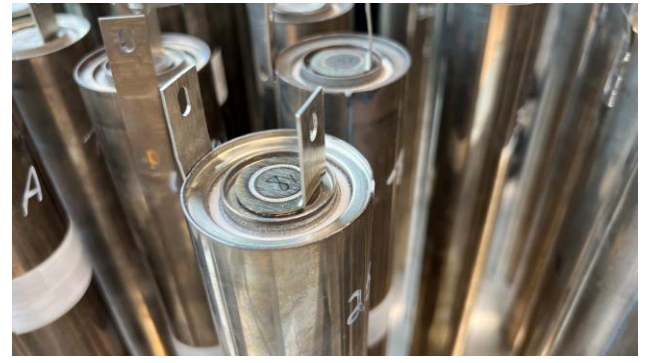
Figure 6 – CERENERGY® cell with positive and negative terminal
