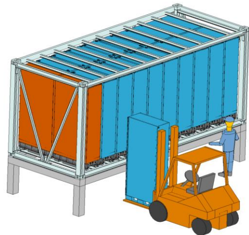
Figure 25 – Assembly 1 MWh GridPack
