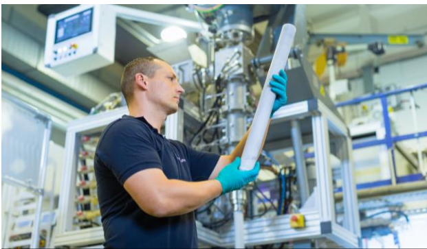
Figure 5 – Ceramic solid state electrolyte at IKTS pilot facility
