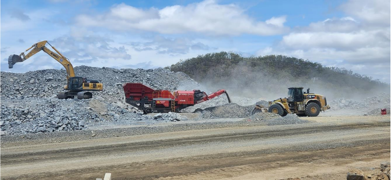
Newly commissioned Terex Finlay Jaw Crusher J-1175 with a 50 tonnes excavator and a CAT 980M preparing the feed on ROM1 Stockpile for the Crushing Plant
