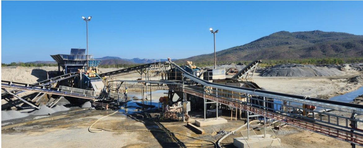
The High-Grade Crushing Circuit on the left, vibrating screen and new Jig on the right, the 6mm fines pipeline at the foreground, pumping fines from the crushing plant straight to the screen.
