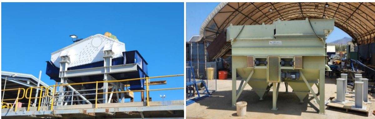
New Schenk Dewatering Screen that will be paired with the new roll crusher (Left); The new Jig being prepared for commissioning (Right)
