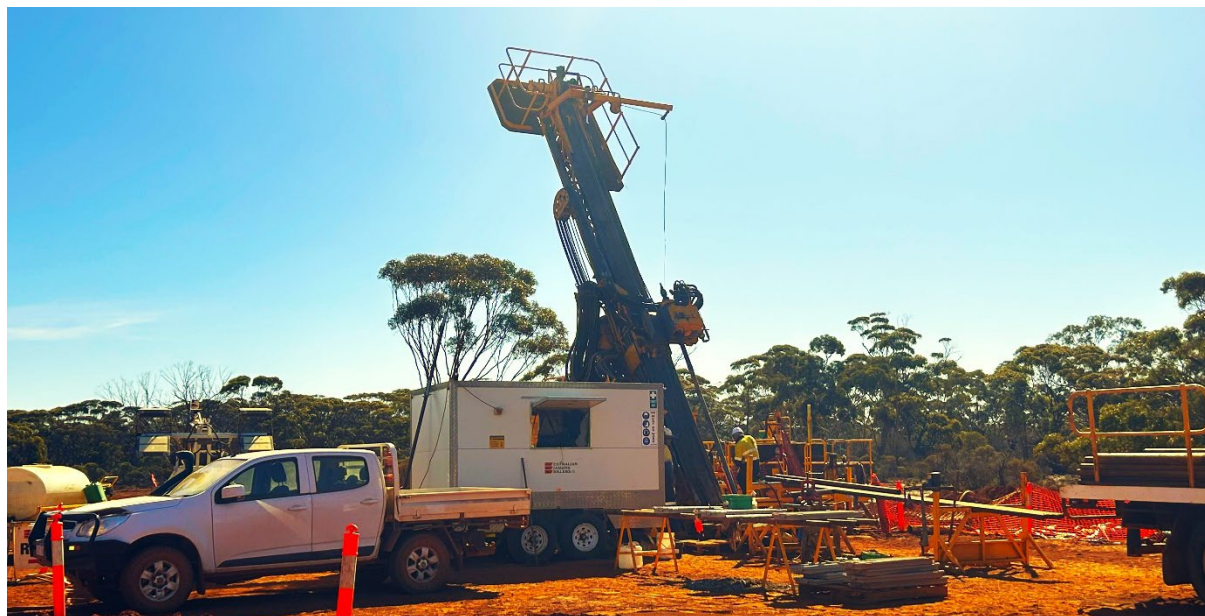
Image 1 – Diamond drill rig at Kamperman (Nov-23).
