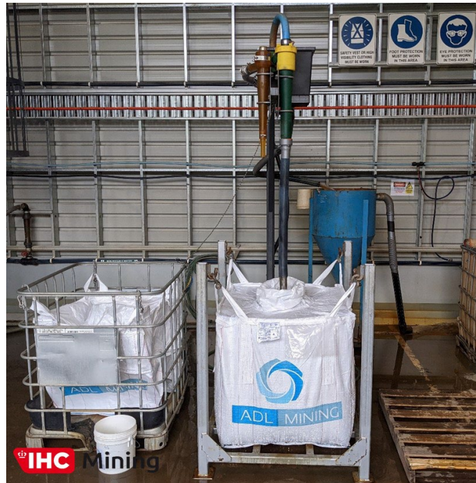
Plate 4 – Slimes removal (material <45\mu\text{m} )
