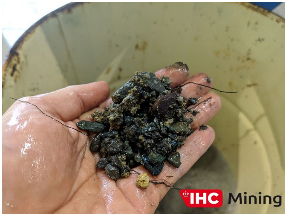
Plate 3 – Pebbles and organic matter from Trommel
