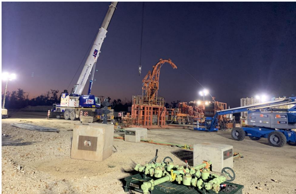
Coiled tubing unit at Daydream-2
