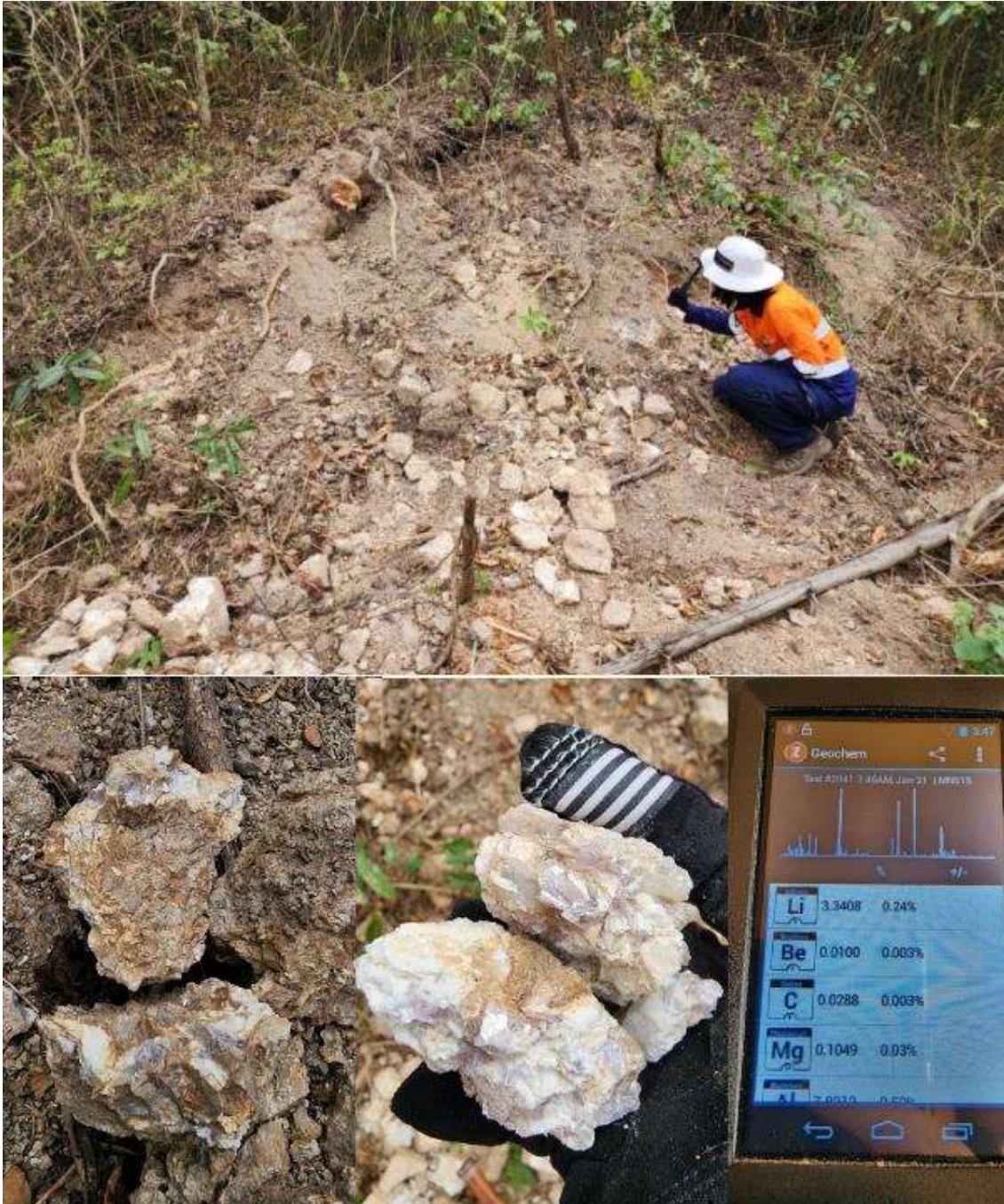
Plate 3: Purple Panther, new pale white-pink lepidolite outcrop at Ratchaburi, 3.34% Li using LIBS
