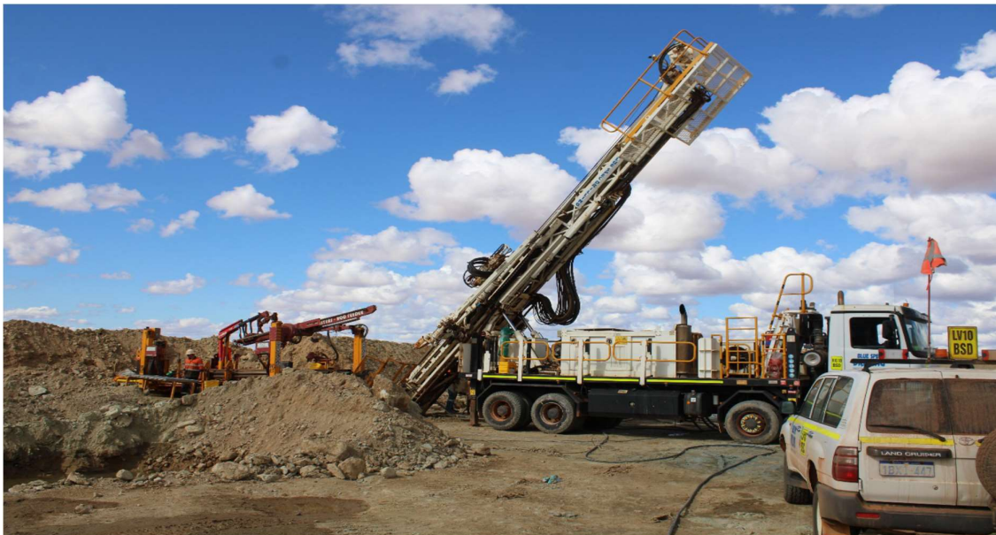
Plate 1: RC drilling rig in operation at the Devon Pit Gold Mine
