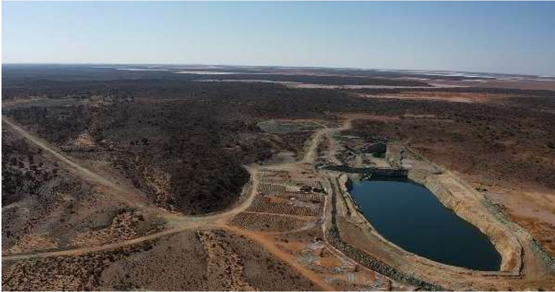
Plate 2: Devon Pit lakes requiring dewatering for mine development (looking north towards Red October and Sunrise Dam gold mines)
