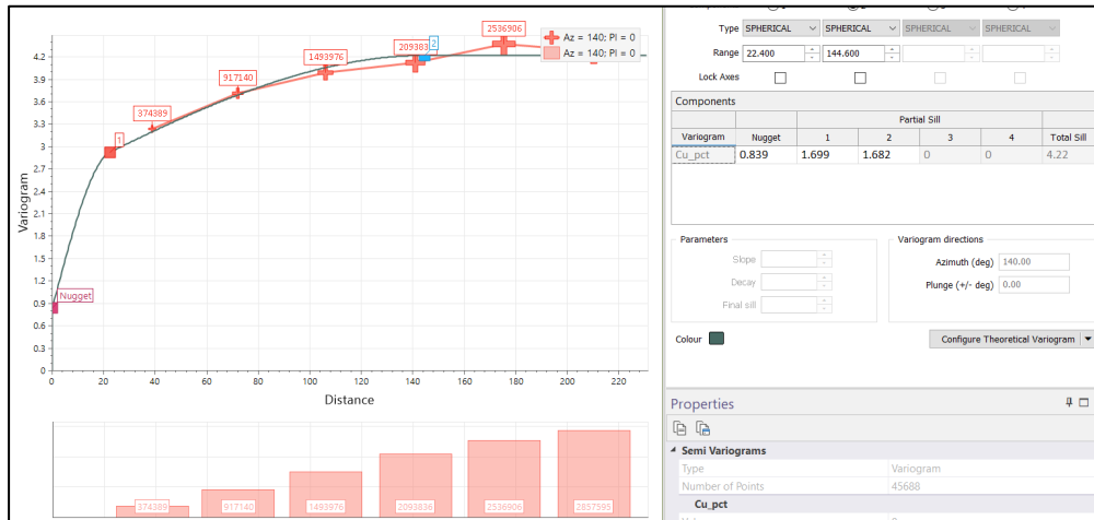
Figure 4-7: FWS Directional variogram, 140° azimuth
