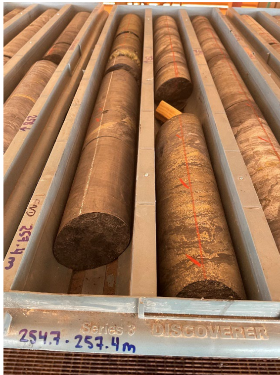
Figure 2-3: 23NFRCDM002 diamond drilled core, ~250m depth
