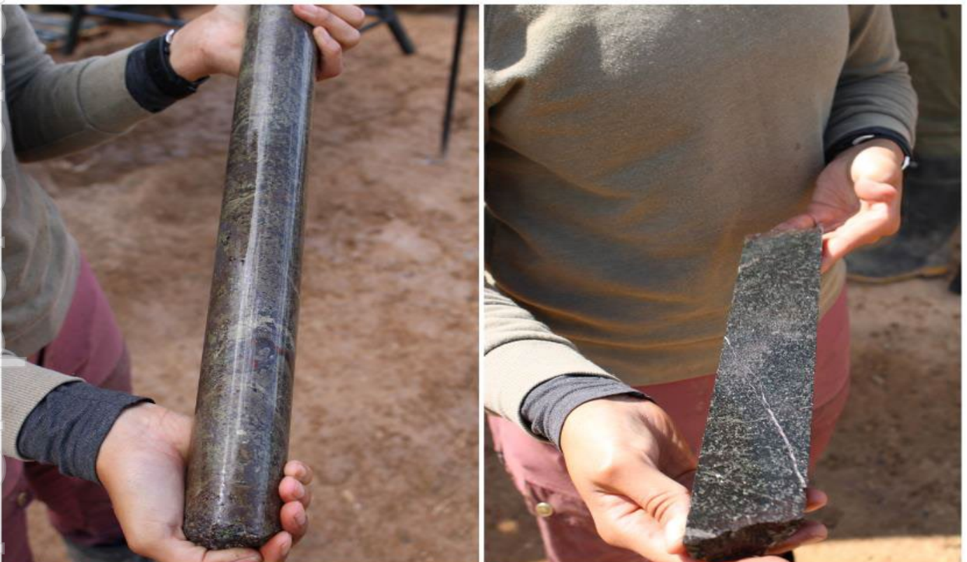
Figure 3: W56 prospect –WL23–367: 21.9m @ 1.02% Ni from 206.65m including 1.35m @ 5.02% Ni from 227.2m and 4.4m @ 1.55% Ni from 247.1m. Massive Sulphides at 227.2m and net texture sulphides at 248.5m, refer ASX on 11 July 2023.
