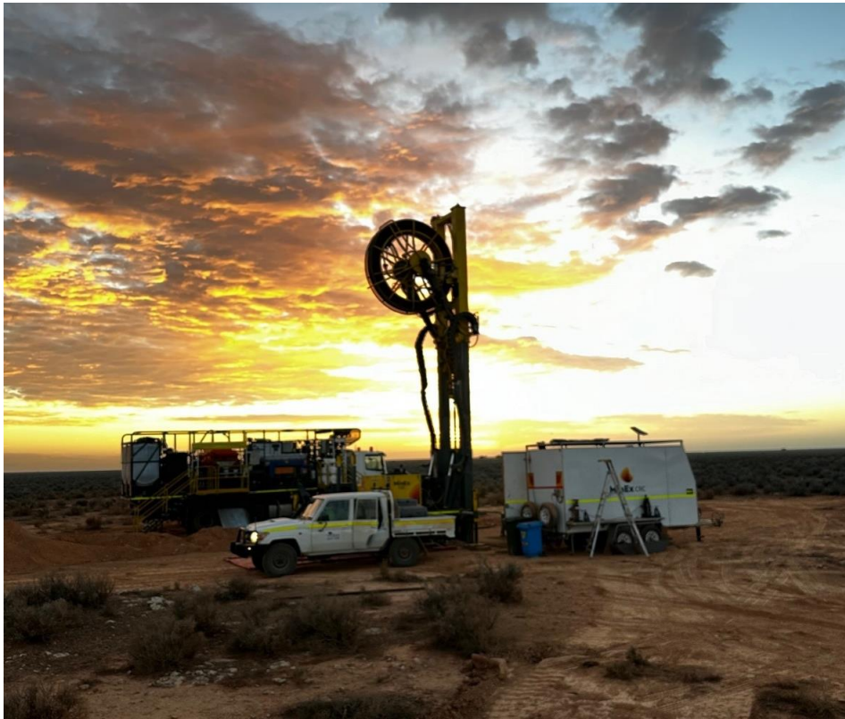
Figure 1: RC Rig on-site at first drill location.
