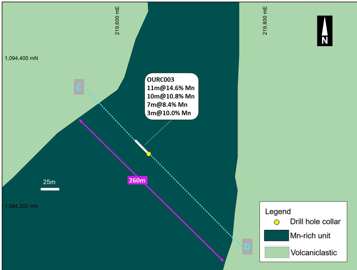
Figure 18: Drill hole OURC003 which intersected 31 metres of manganese in the 50 m hole – section line shown in blue
