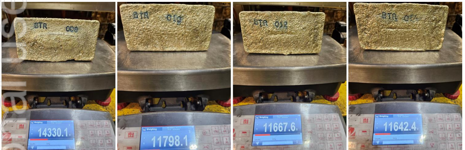
Figure 2 – Example weights of gold doré bars BTR008, BTR010, BTR012, BTR014
