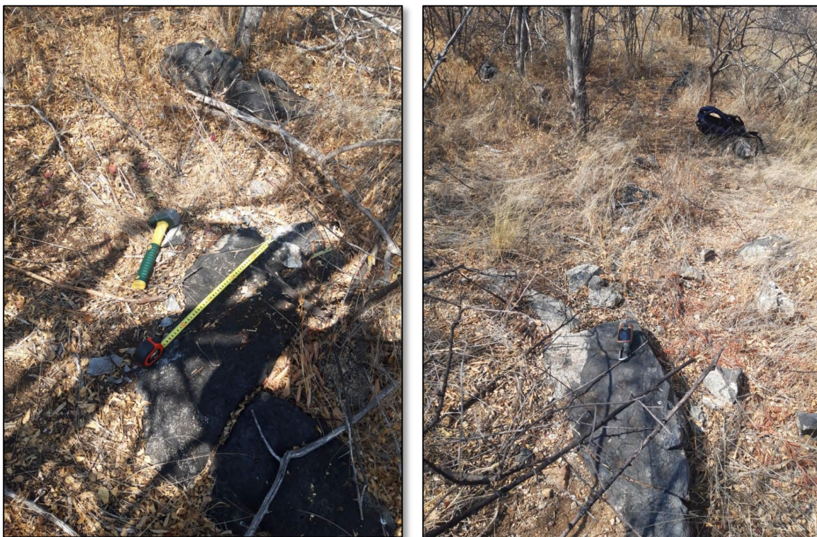
Figure 3: Niobium bearing dyke KMRC0300 showing width and outcrop at two sites. Note the ground slope and thick regolith and vegetation cover obscuring much of the area.
