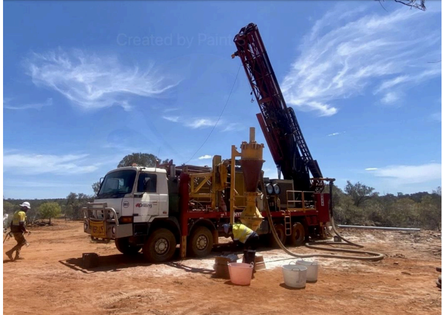
Photo 1: Drilling rig at Ethel Maude Mine, collecting samples for assay.
