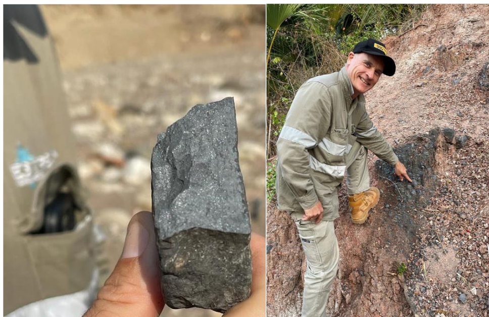
Figure 2: (R) Platy Pyrolusite forming >90% of a specimen found during field reconnaissance to the exploration concessions. (L) Sub-cropping manganese mineralisation in hillside scree of the Bobonaro Formation within Concession ZA-01
