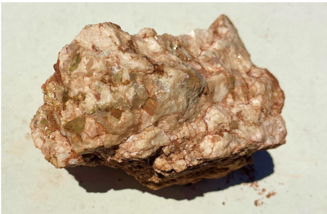
Figure 5 - Fractionated pegmatite from Carr Boyd East containing Albite (70%) + Quartz (25%) + Rb Muscovite (5%) and Zinnwaldite (trace %) 8
