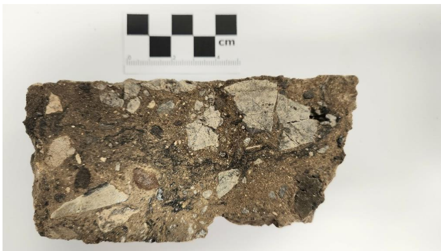
Figure 13 MJLLDD016 Polymict breccia in the brittle zone
