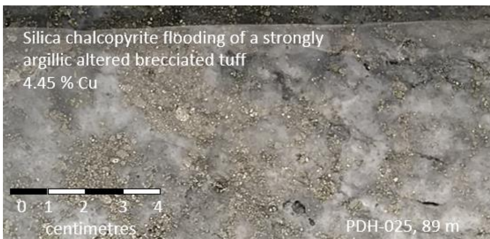
Figure 3-2. Advanced Argillic Alteration, veinlets of chalcocite and fine sulphides. (MA 2024)
