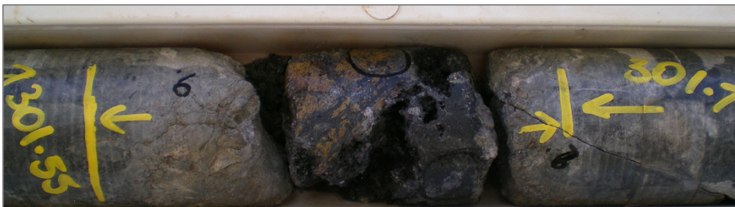
Photo 1 – Vein of massive sulphide from 301.6m in EPT062 at the BM5 prospect
