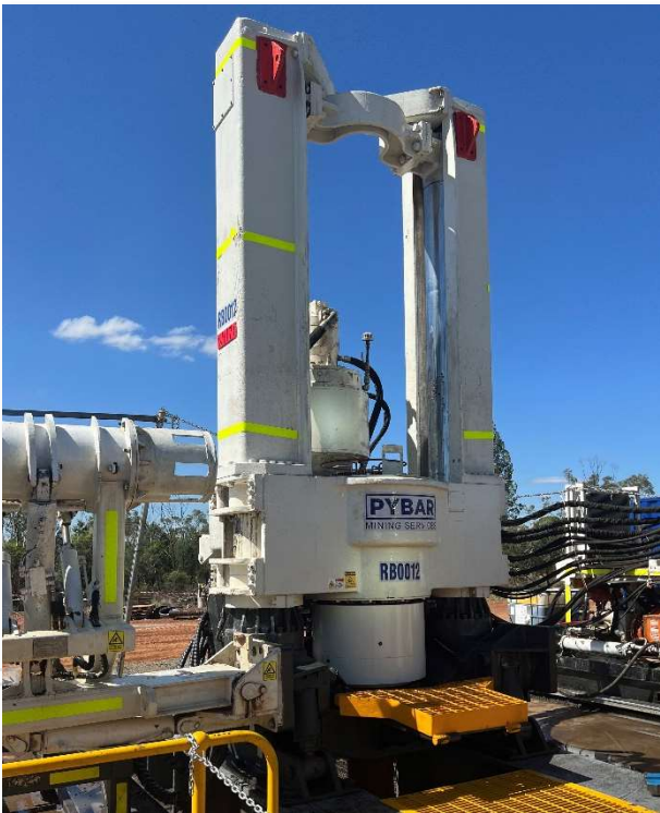
Figure 1: Pybar raisebore rig in place reaming
