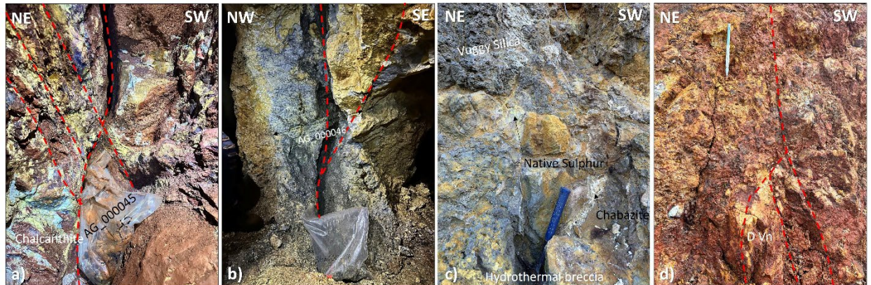
Figure 10. Bourbon workings. a) D-veins, alteration Ser + kao, Hem < 30%. b) Alteration Ser + Kao, secondary Cc <10%, Cpy + Py, Cv <3%. Bourbon prospect on surface. c) Hydrothermal breccia with alteration of vuggy silica + Ser + Kao, presence of native sulphur, Calcantite, Py diss < 25%, chabazite veins filling open spaces, this rock chip sample yielded AG_000024 0.5m x 0.5m@ 40 g/t Au. d) alteration Ser + Kao, Hem <40% diss, D-veins.
