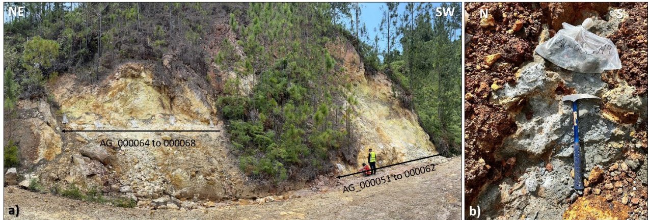
Figure 20. a) Systematic channel rock sampling at the Arabica prospect. b) Quartz porphyry outcrop with advanced argillic alteration, disseminated Py <50% + Cpy, located 450m SSE of systematic rock sampling.
