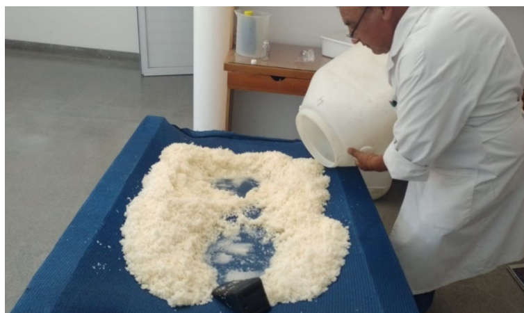
Figure 9: Salt Precipitation Stage, with concentrated brine separate from Salts
