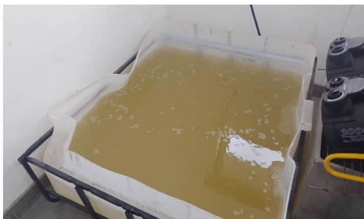
Figure 8: Primary Evaporation Stage of Solaroz Brines
