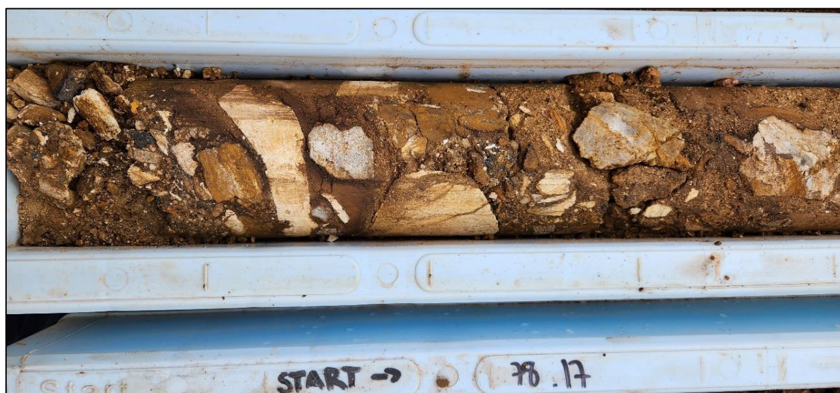
MLJDD020_178.0m_Polymictic Breccia with silica-pyrite clast
