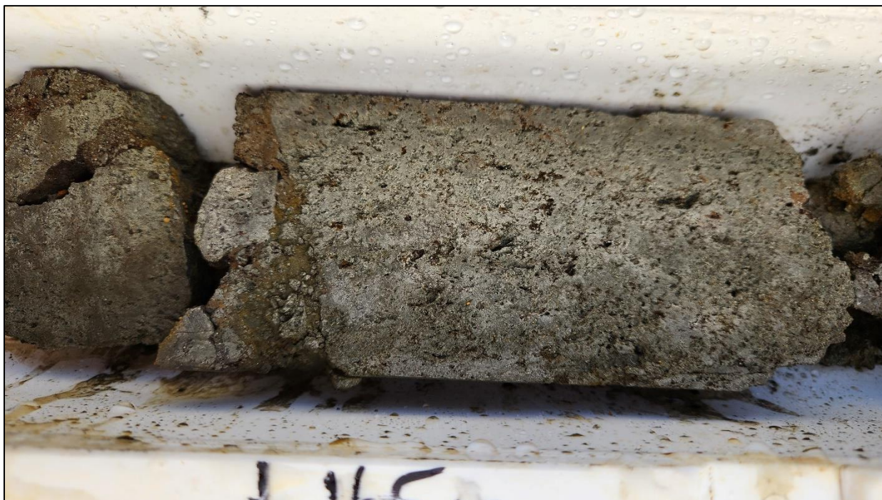
MLJDD018_164.5m_Massive pyrite in Breccia
