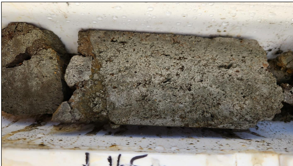
MLJDD018_164.5m_Massive pyrite in Breccia
