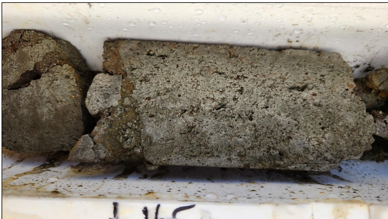
MLJDD018_164.5m_Massive pyrite in Breccia
