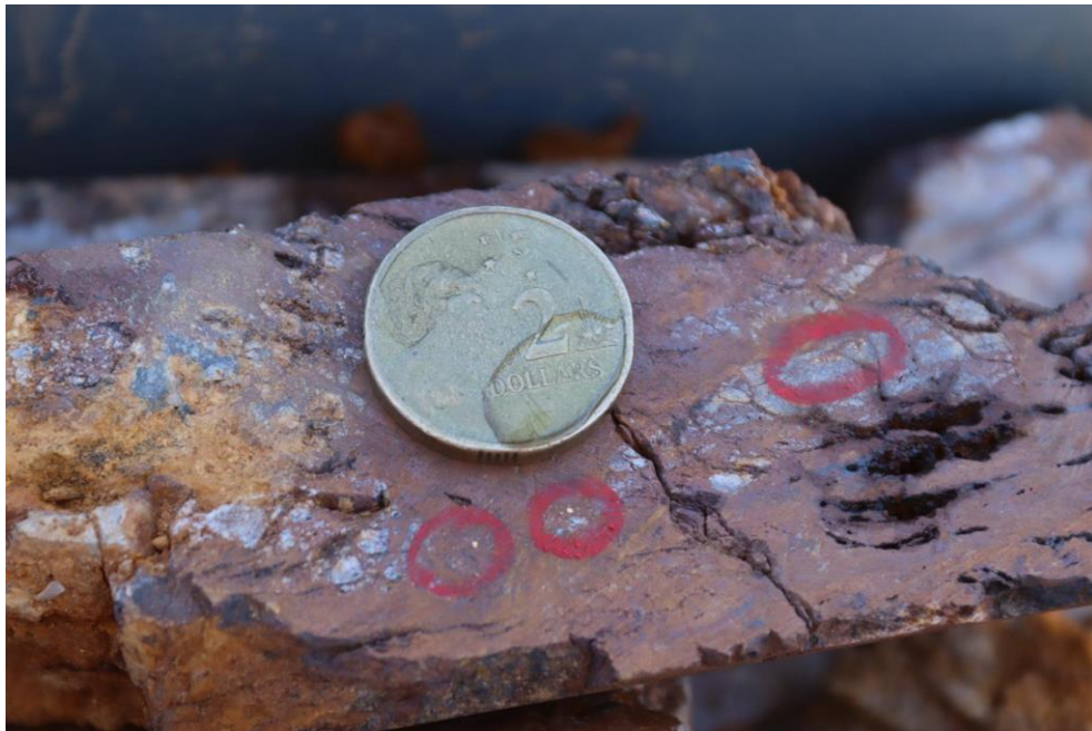
Figure 1 - CTWMET003 at 54.05m, showing visible gold (VG, circled) with $2 coin (20.5mm diameter) for scale
