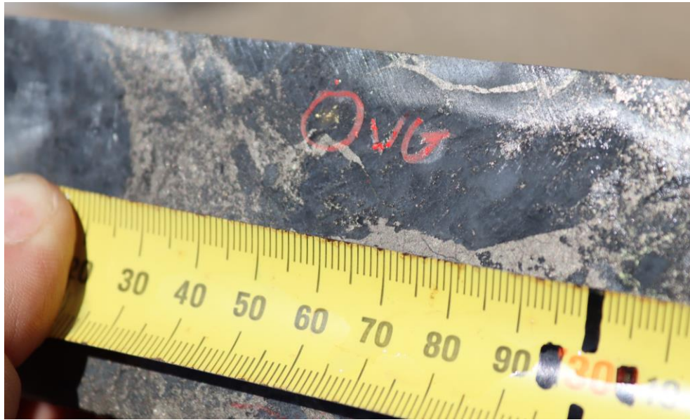
Figure 2 - CTWMET001 at 138.75m, showing visible gold (VG, circled) with tape measure for scale
