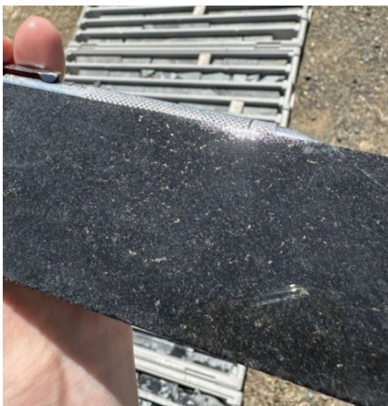
Figure 1. Drill hole EFO7D (10m at 1.2g/t 3E PGE from 388m) showing disseminated interstitial Ni-Cu-Fe sulphides (yellow) in diamond drill core at 397.8m (left) and photomicrograph (field of view 1mm across) of the mineralisation (composed of bronze pentlandite, yellow chalcopyrite and brown pyrrhotite).
