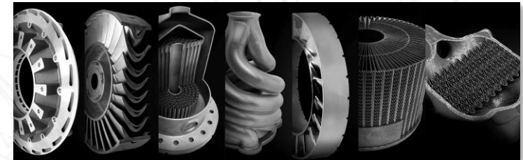
Additive manufacturing (complex geometries and housings)
