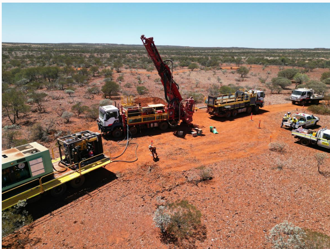
Figure 1: RC Rig on-site at first drill location.
