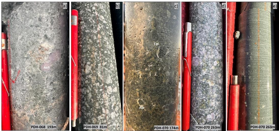
Figure 6. a) diatreme with anhydrite + illite + sericite alteration. b) diatreme with secondary biotite + albite alteration. c) diatreme with alteration of Epidote. d) Diatreme with alteration of albite + Epidote. e) fresh andesite dam.
