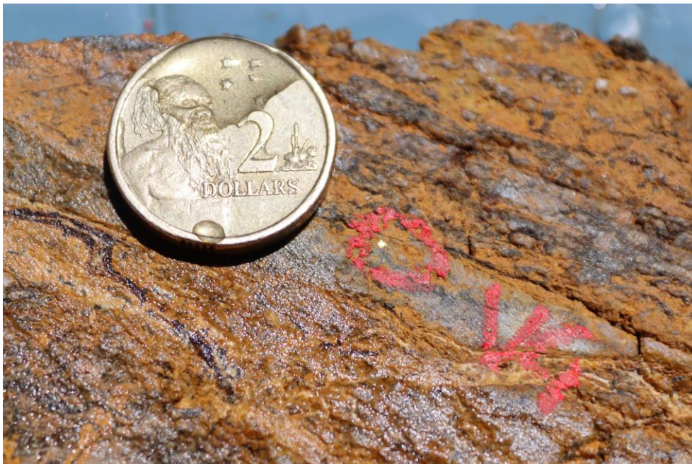
Figure 1 - CTWMET004 at 71.85m, showing visible gold (VG, circled) with $2 coin (20.5mm diameter) for scale
