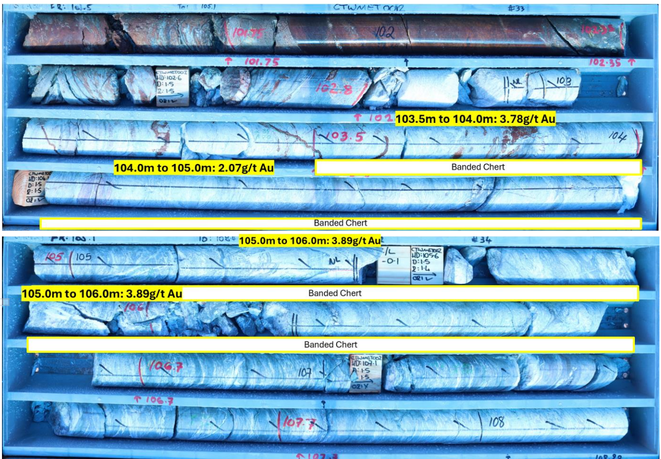
Figure 8 - CTWMET002 Trays 33 & 34 showing mineralised intercept of 3.2m at 2.62g/t Au in chert unit
