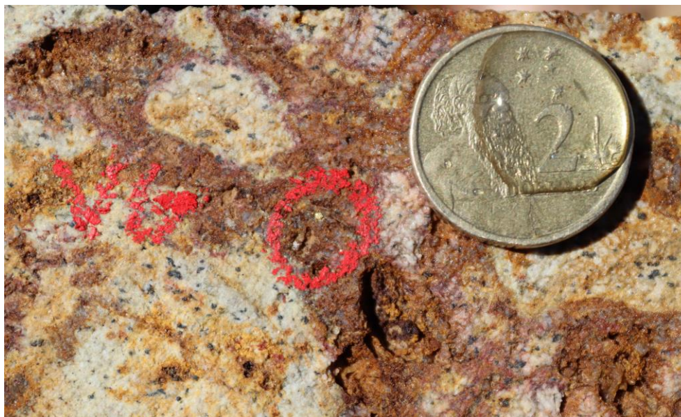
Figure 2 - CTWMET004 at 48.80m, showing visible gold (VG, circled) with $2 coin (20.5mm diameter) for scale
