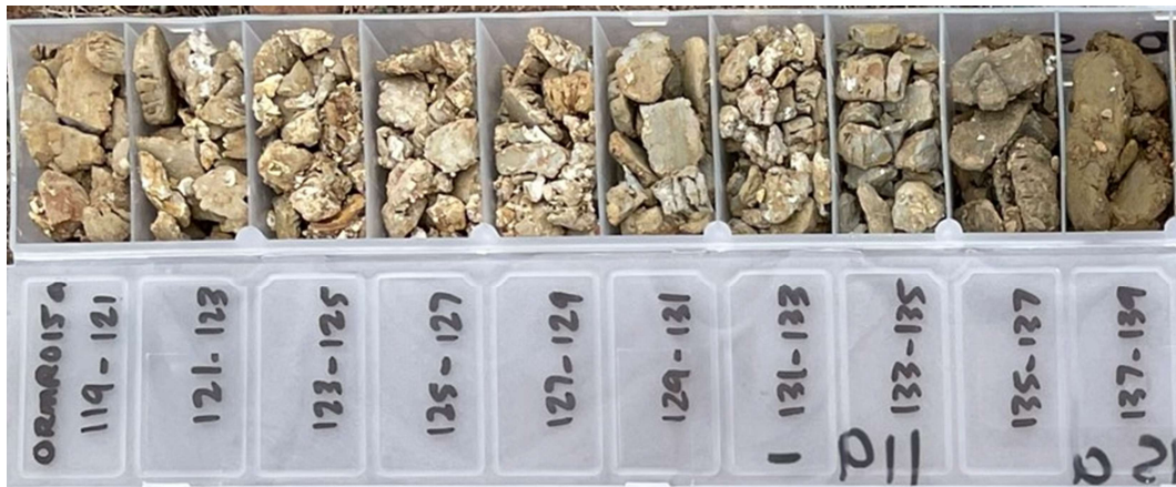
Image 1 – Drill samples from ORMR015A showing the kaolinitic clay marker unit from 121-130m and floodplain silt from 130-137m.
