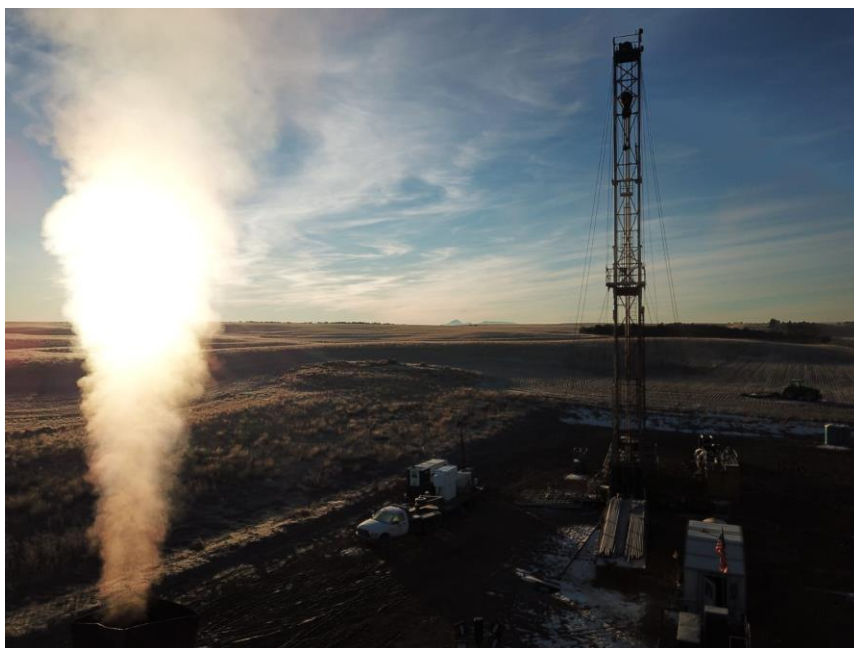
Figure 1: Jesse-1A flare-stack venting reservoir gas and helium at a rate of 1mmcf 1
