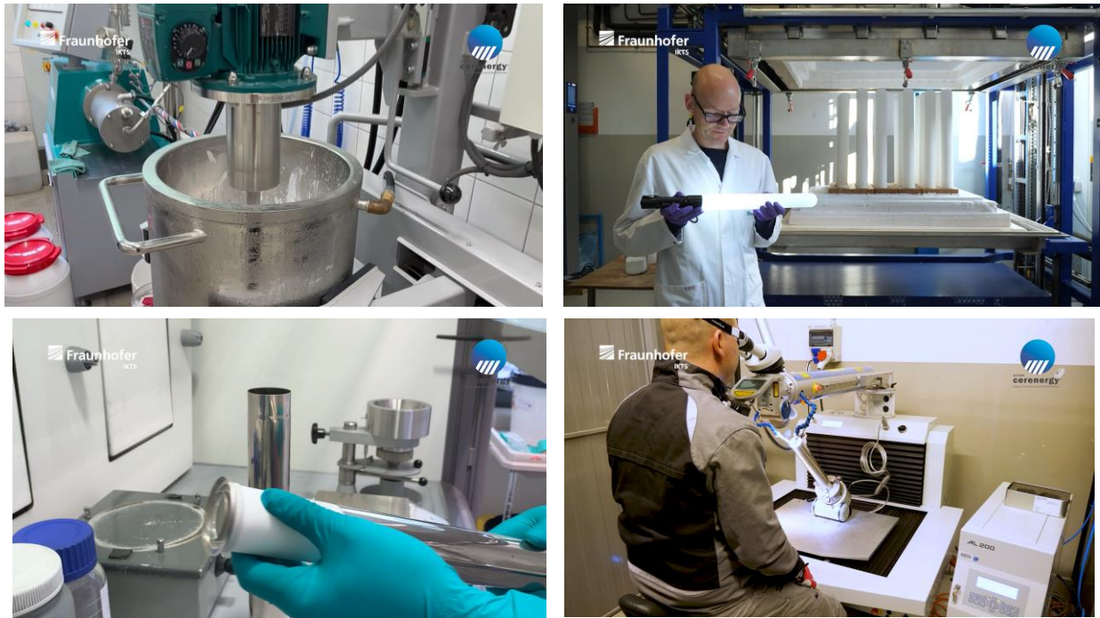
Figure 2 – Production of battery cells at Fraunhofer IKTS Hermsdorf pilot plant facility
