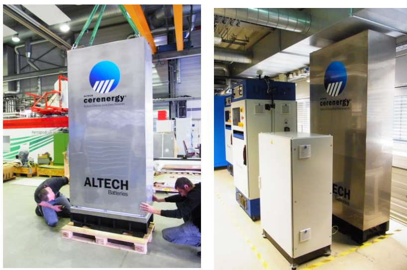
Figure 4: Delivery of the battery casing and heat loss testing at Fraunhofer IKTS Dresden
