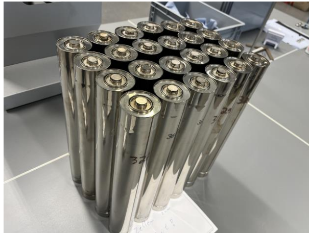
Figure 3 – Some of the completed battery cells waiting performance testing
