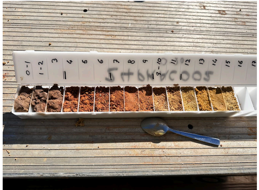
Figure 3: Parrakie aircore drilling Loxton/Parilla Sands (left) and clay/clayey sands intersected in the drilling
