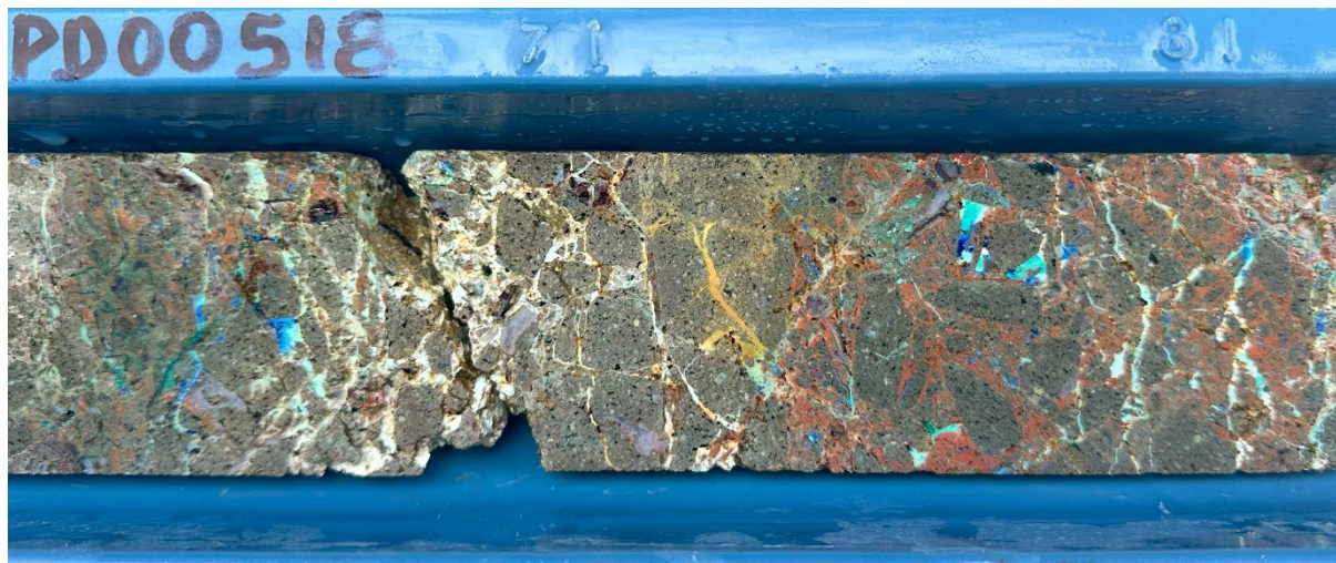
Figure 1: Example of secondary copper mineralisation at 75.40m depth in 23PCCD0002
