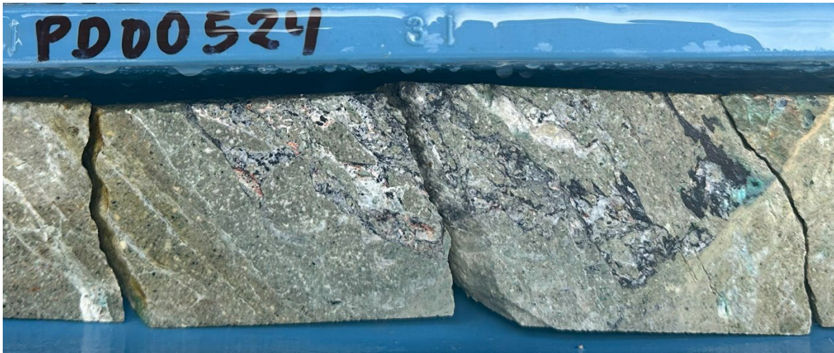
Figure 6: Example of copper mineralisation (chalcocite) at around 82.45m depth at Cumbre Coya Target 23PCCD0002
