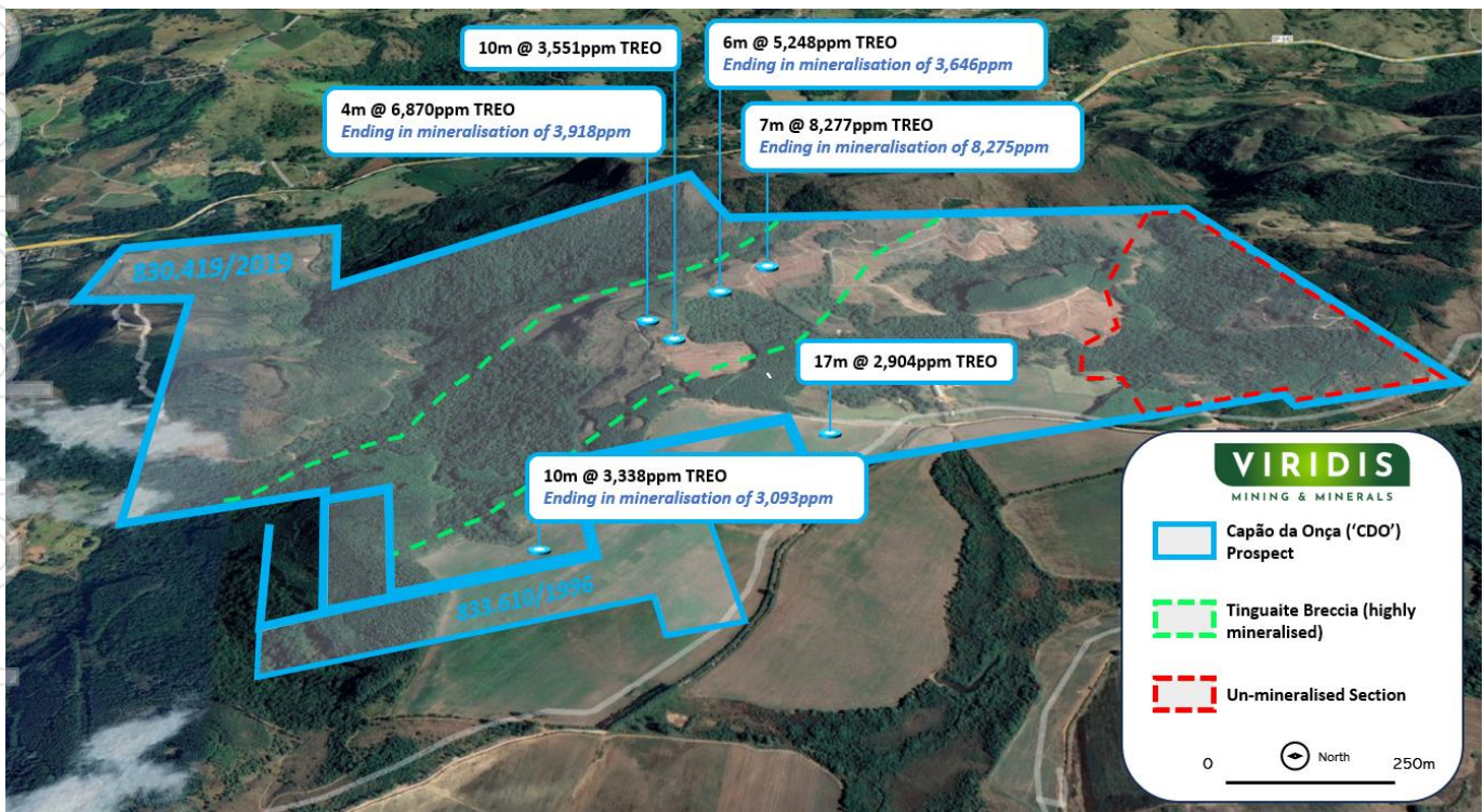
Figure 4: Satellite view of Capão da Onça which highlights interpreted corridor of significant high-grade mineralisation and area of concession which remains un-mineralised in economic levels of TREO (~<800ppm).
