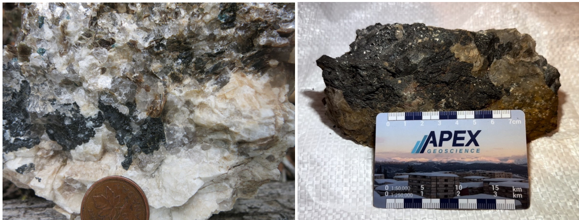
Figure 12: Left: Pegmatite with minerals of feldspar (white/cream), quartz (clear), tourmaline (black), muscovite (bronze), and apatite (blue). Right: Black tourmaline crystals in pegmatite.
