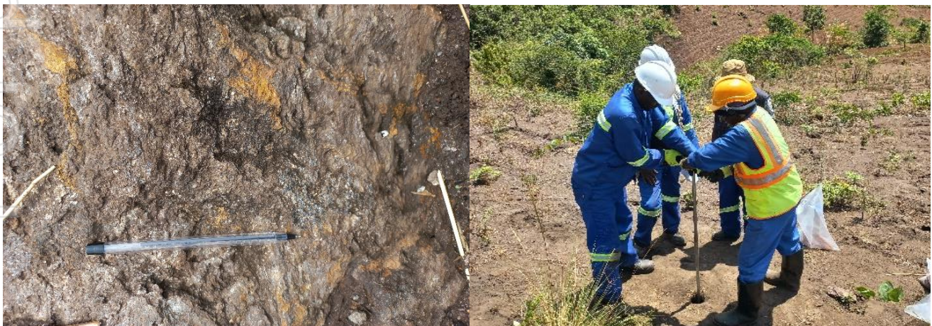
Figures 4 & 5: Graphitic gneiss outcrop (left) and NGX team hand auger drilling (right)
