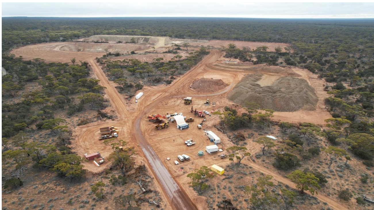
Figure 1. Jeffreys Find Mine Site at completion of the stage 1 pit – note Run of Mine ore stockpiles lower right.
