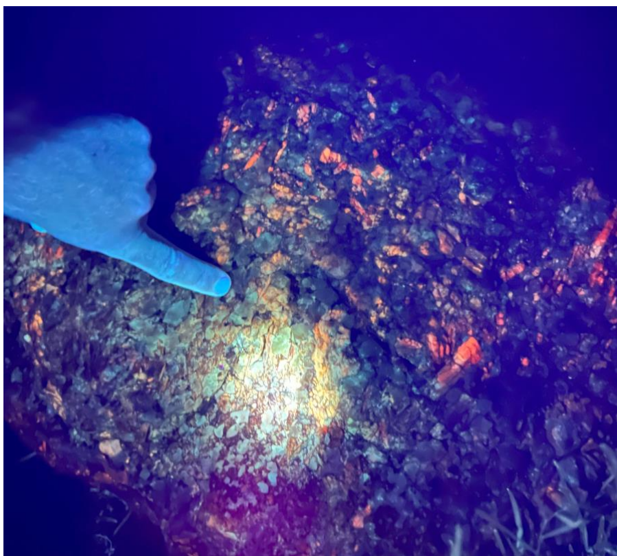
Figure 1: Outcropping spodumene (Orange) rich pegmatite from sample location 23WS0044.
