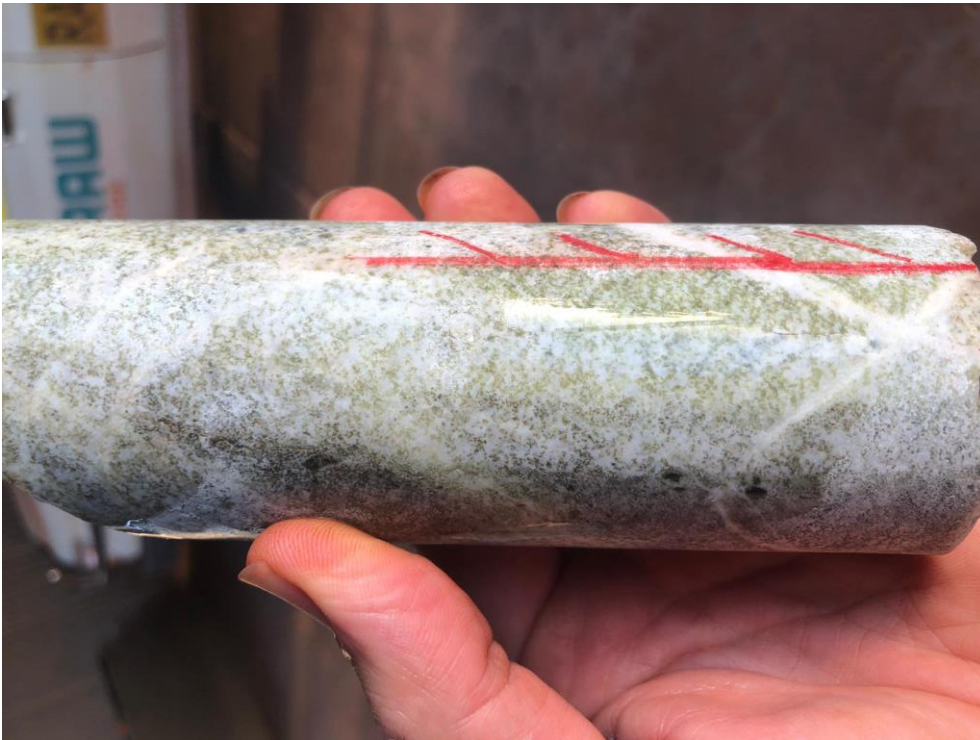
Figure 6. Bleached and altered zone with calcic-sericitic-epidote alteration in OND001 (Coral Bug prospect).
