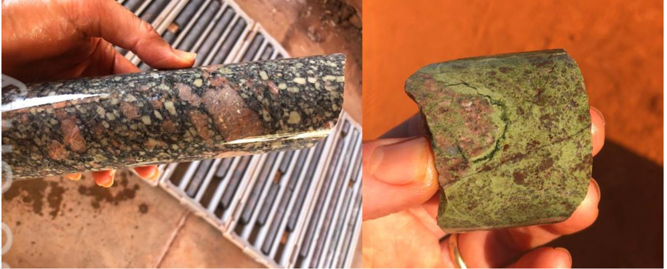
Figure 8. Examples of alteration in OND002 (Hammerhead prospect) including (left) variable mylonite alteration and (right) epidote-hematite alteration
