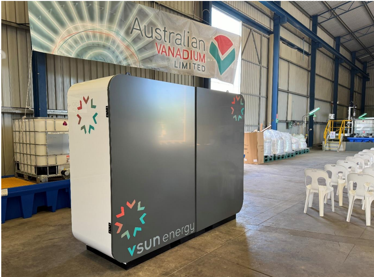
Figure 4 - VSUN Energy prototype residential vanadium flow battery
