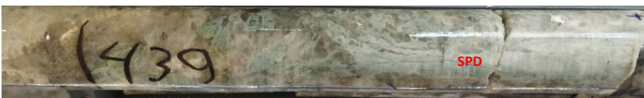
SADD223: 435.35m (1.63% Li 2 O). Green spodumene associated to quartz, feldspar and mica.
