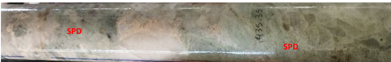
SADD223: 435.35m (1.63% Li 2 O). Green spodumene associated to quartz, feldspar and mica.
